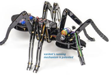
Once variAnt is built, the pre-assembled and upgradable Code Modules enable quick and easy access to the Arduino Programming.
