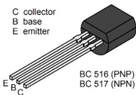
With a voltage between the base and emitter of about  $U_{BE} = 0.7 \text{ V}$  ( $\text{V} = \text{Volt}$ ), a transistor reduces the resistance between collector and emitter and switches through.
