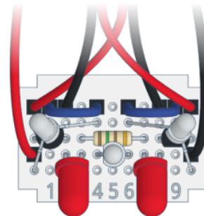
For this function, it is especially important to use very uniform lighting. In order for varikabi to turn around repeatedly, the tilt of the sensors must be very well adjusted.
