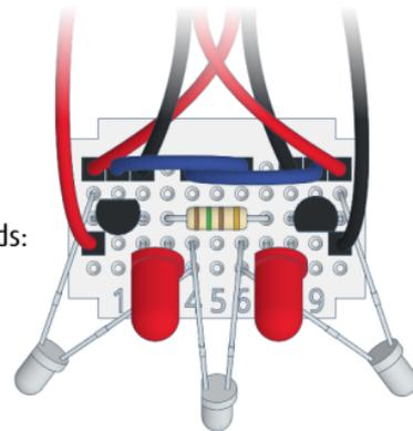
Adjust the distance of the side sensors to the size of the object. Experiment with the tilt of the sensors so that both following and stopping work well.
