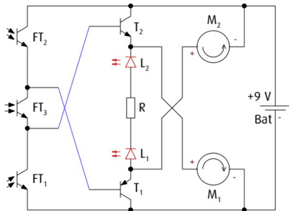
In brake mode, the LEDs are now reverse-poled between the transistors. However, they can still light up. When both transistors are blocked, the LEDs are powered by the stationary motors.
