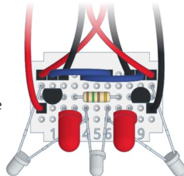
Adjust the tilt of the side sensors so that varikabi always turns in time at the edge. Adjust the tilt angle of the middle sensor so that varikabi stops at bright surfaces.
