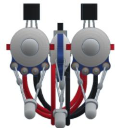
Adjust the distance between the side sensors to the line width. Experiment with the inclination of the sensors so that varikabi comes to a standstill at the end of the line.
