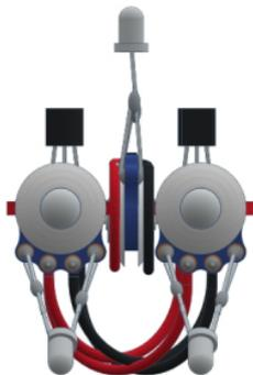
The ambient light should not be too strong for this function so that varikabo can recognize the light well. Experiment with the distance and inclination of the side sensors.
