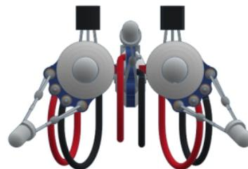
Adjust the inclination of the side sensors so that varikabo always turns on time at the edge. Adjust the tilt angle of the middle sensor so that varikabo stops on a light-colored surface.
