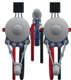
Adjust the distance between the side sensors to the size of the object to be tracked. Adjust the tilt angle of the middle sensor so that it is only slightly above the object.
