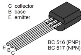
With a voltage between the base and emitter of about  $U_{BE} = 0.7 \text{ V}$  ( $V = \text{Volt}$ ), a transistor reduces the resistance between collector and emitter and switches through.
