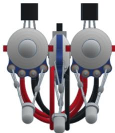
Adjust the distance between the side sensors to the line width. Experiment with the inclination of the sensors so that varikabo comes to a standstill at the end of the line.
