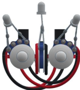
If you place varikabo on the floor at some distance from the lamp, it will move quickly towards the light. The inclination of the sensors must be well adjusted so that varikabo always turns back.
