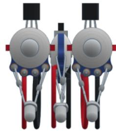
Experiment with the distance between the side sensors and the inclination of the center sensor to adjust the speed control as well as possible.
