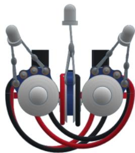
If you place varikabo on the floor at some distance from the lamp, it will move quickly towards the light. The inclination of the sensors must be well adjusted so that varikabo always turns back.
