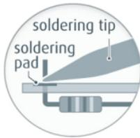
4. Now add solder between the solder pad, the component wire and the soldering tip without removing the soldering tip. Use only enough solder to cover the entire solder pad.
