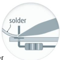
5. Stay with the soldering tip at the soldering point for about one second until the used solder is well distributed, so that a shiny silver cone appears around the wire.
