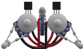
The further down you point the side sensors, the closer varikabo moves to obstacles. The middle sensor must be positioned slightly above the obstacles.
