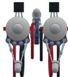
Adjust the distance between the side sensors to the size of the object to be tracked. Adjust the tilt angle of the middle sensor so that it is only slightly above the object.
