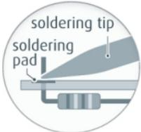
4. Now add solder between the solder pad, the component wire and the soldering tip without removing the soldering tip. Use only enough solder to cover the entire solder pad.
