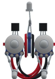
The ambient light should not be too strong for this function so that varikabo can recognize the light well. Experiment with the distance and inclination of the side sensors.
