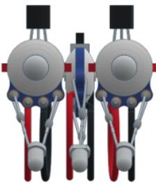
Experiment with the distance between the side sensors and the inclination of the center sensor to adjust the speed control as well as possible.
