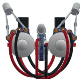
The further you point the middle sensor upwards, the closer varikabo moves to the lamp. If you hold your hand between the lamp and varikabo, it will try to get back into the light.
