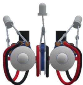
For this function, it is particularly important to use very uniform lighting. The inclination of the sensors must be very well adjusted so that varikabo always turns back.
