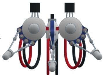
Adjust the distance between the side sensors to the size of the object. Experiment with the inclination of the sensors so that both following and stopping work well.
